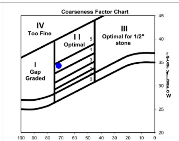
**Fig 1b: Coarseness and Workability Chart for Mix Design with Reduced Cementitious Content**
