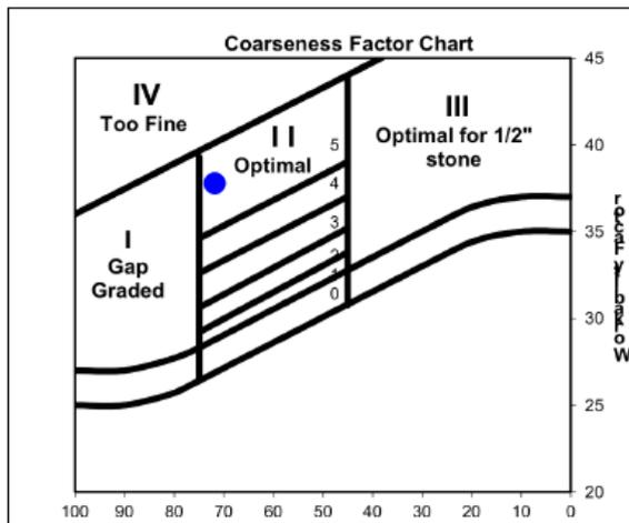
**Fig 1a: Coarseness and Workability Chart for Original Untreated Mix design**
