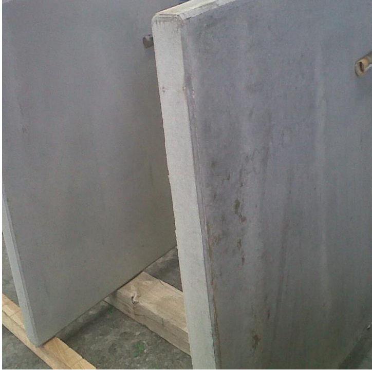
Fig 10. This application was done at a Precast concrete facility that was having an issue with there supply water. The element of the Left had CAM 110 in the mix water during batching and the element on the right did not.
