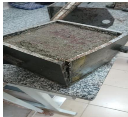
Fig 2b: Pressure test cracked the form not the concrete.
