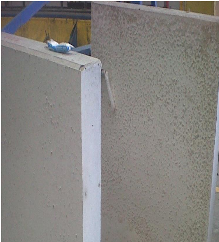
Fig 11. Same elements from another angle, it readily apparent the quality improvement in visual effect, not to mention the internal improvements of performance of the concrete.
